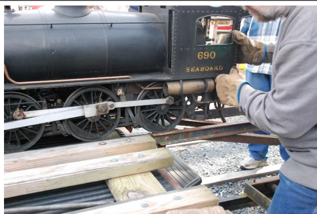
After carefully aligning the transfer table for height, the live steam ten wheeler, weighing some 650 pounds, is moved from a pickup truck bed to be mated with its tender.
