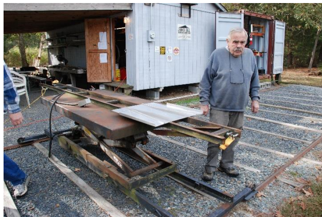
An ingenious transfer table can be adjusted for height to transfer locomotives and rolling stock from the storage container (right rear of photo) or from a vehicle used to transport the model.
