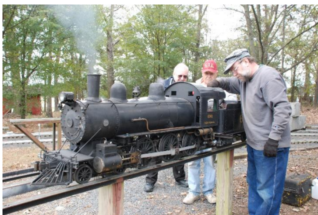
The owner is firing up his live steam 4-6-0. The locomotive is fired by coal, and boiler operating pressure is over 100 psi. It took about 40 minutes to get the boiler up to operating pressure.
