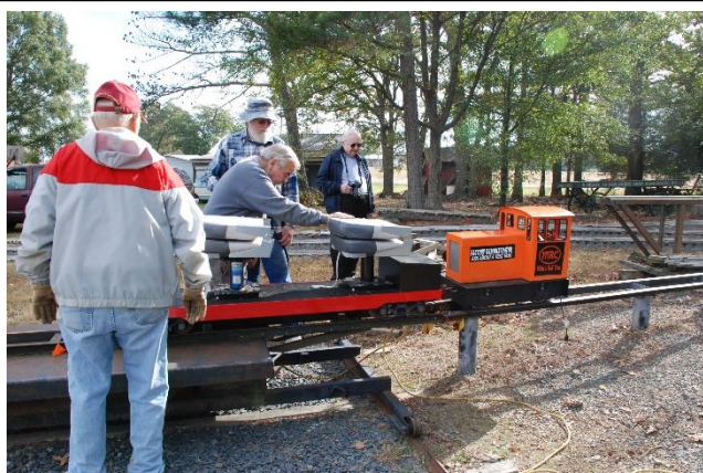
The transfer table in use as a locomotive and ride-on flatcar are moved onto the railroad's loading track. The loading track goes downhill to the right and merges in with staging tracks.
