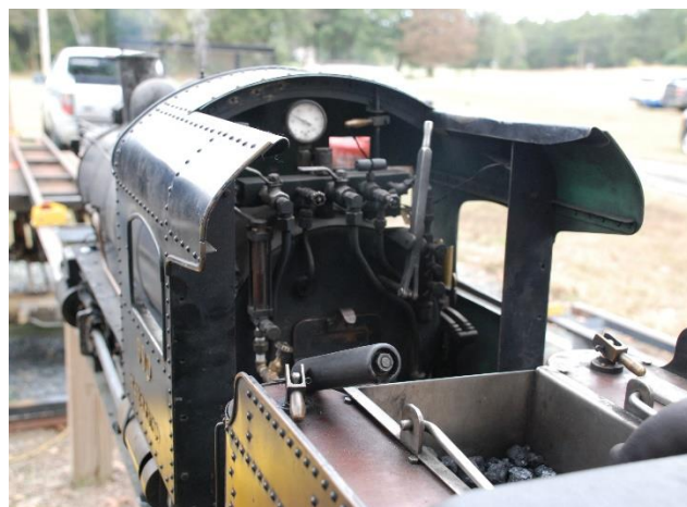
Real functional backhead details! The tender can carry enough coal and feedwater for about 3 hours of operation.
