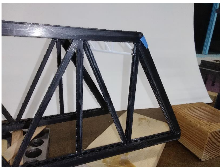
Photo 5: An asymmetrical panel was added to one side of the bridge to create the skew for the modified single-track bridge.
