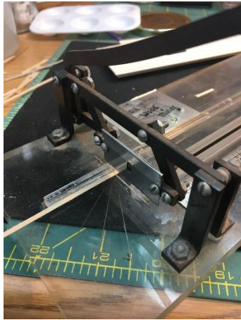
Pic 6: A Shay Wood Miter Tool that cuts by slicing, not chopping, which gives you a much more precise cut.
