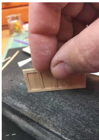
Pic 12: Carefully sand the edges of the door checking to make sure they are smooth.
