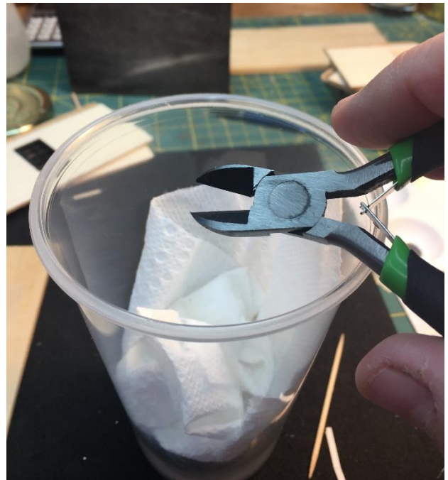
Pic 21: Use safety glasses when cutting the pins! The cup and wadded paper towel are used to catch the bouncing part and the sharp flying pin.
