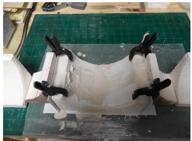
Pic 9: With styrene dams in place, plaster was poured into the resulting cavity.
