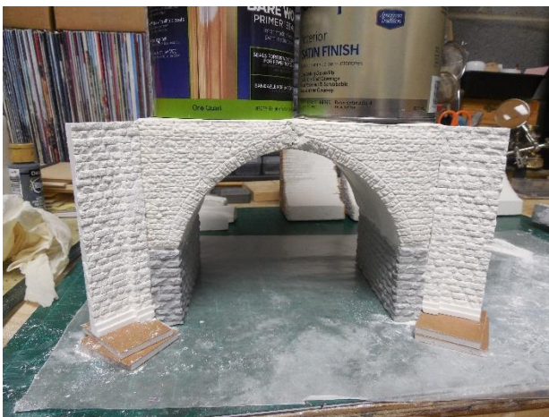
Pic 10: Cast piers and wing wall sections are assembled.
