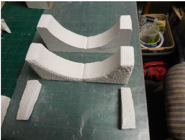
Pic 8: The assemble arch was cut in half to allow widening for double track.
