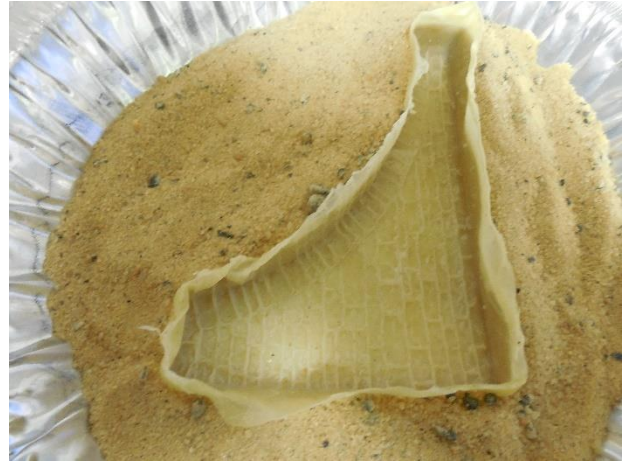
Pic 5: The completed latex mold is ready to pour sections of stone for abutments and extensions.
