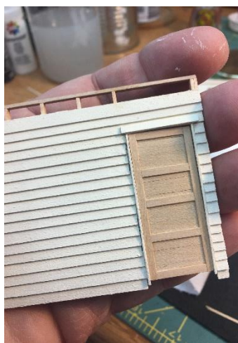
Pic 13: Test fit the door to the frame, re-sand and fit as necessary.
