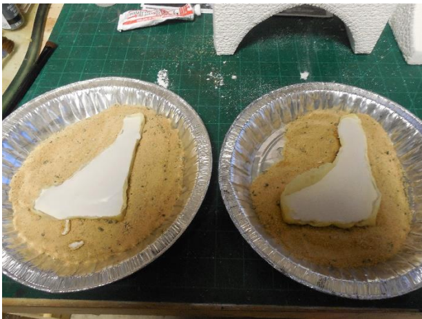
Pic 6: The latex molds are filled with hydrocal. Just waiting for it to set up.
