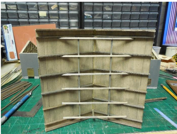
Pic 7: A view of a completed roof structure with rafters and collar ties in place.
