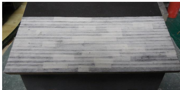
Pic 9: Roof panel with overlapping tape applied as tar paper strips.
