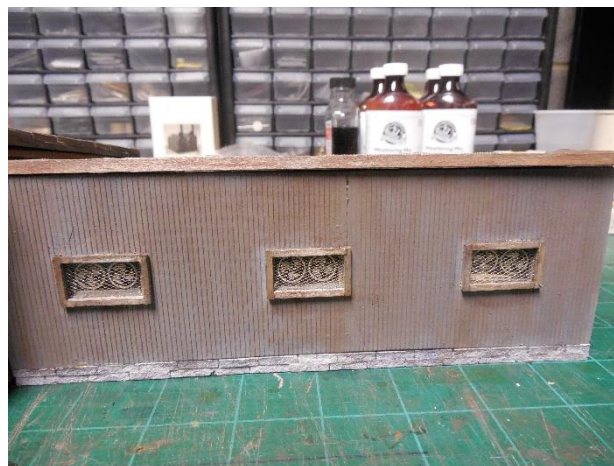
Pic 26: Cooling room assembled, fans installed, painted and weathered.
