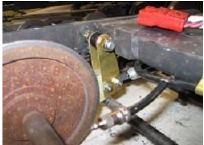
Truck with air brake hardware installed.
