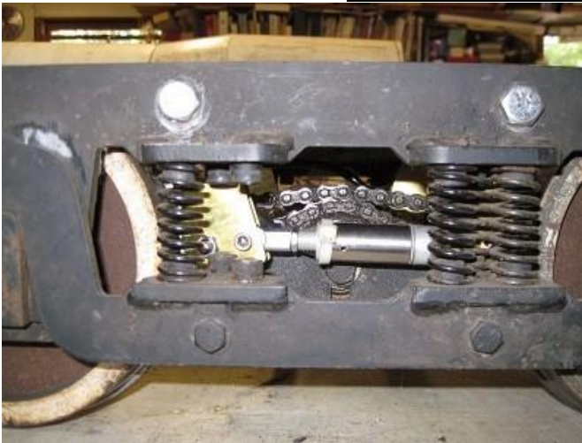
Truck side frame with air brake air cylinder visible.
