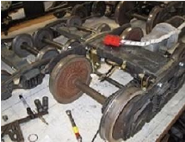
Truck with air brake hardware installed.
