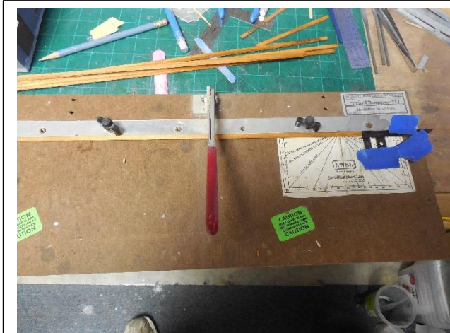
Pic 19: NWSL Chopper III makes it easy to cut repetitive pieces for scratchbuilding.
