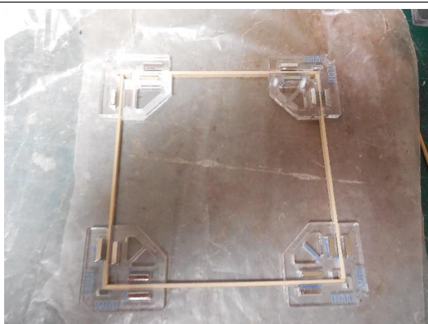
Pic 15: Perimeter of a floor framing system clamped with magnetic clamps to keep square.
