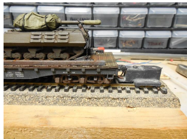
Pic 7: Couplers and/or trucks are shimmed to ensure correct height of Kadee couplers.
