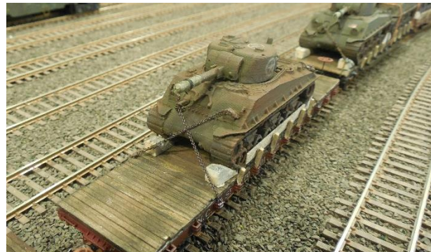
Pic 14: Typical tank tie-downs.
