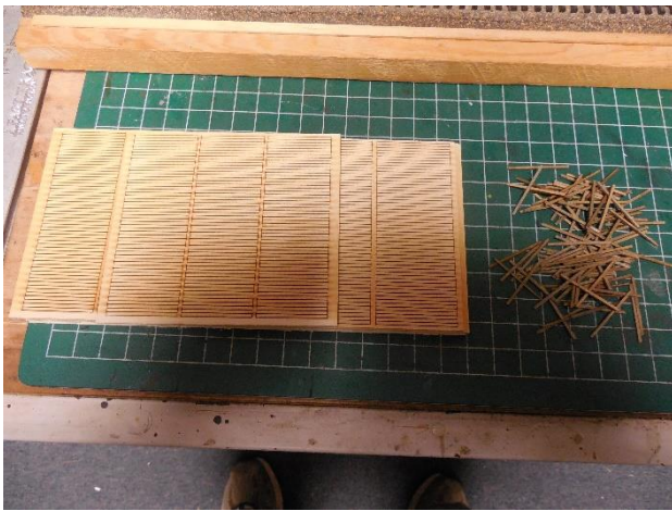
Pic 4: Sheets of laser cut 2x6 lumber are cut to length
