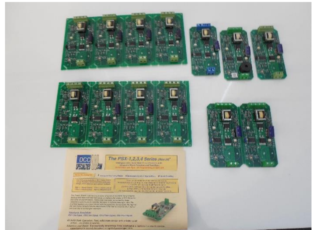
Pic 5: PSX boards in various configurations will be used for current protection in each district.
