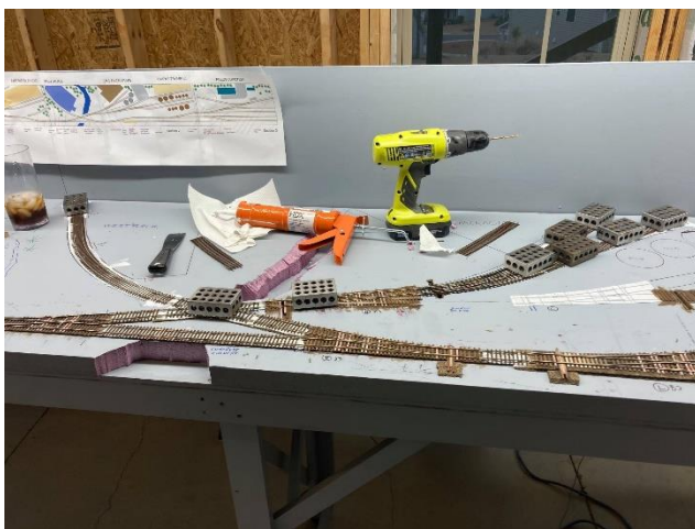
Scott Perry's trackwork installation is progressing well. Lots of 1-2-3 blocks holding track in place while adhesive dries. Photo from Scott's Facebook Post.
