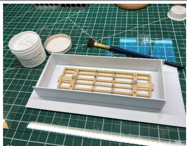
Pic 19: Build mold dam and add mold release.
