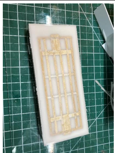
Pic 26: After curing, remove the mold from the mold dam.
