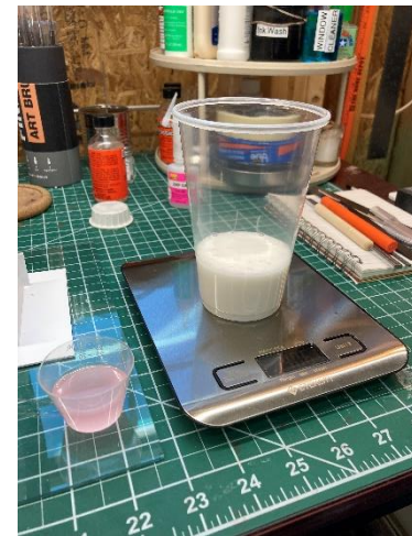
Pic 23: Measure and mix the silicone and activator.
