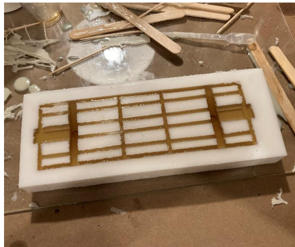
Pic 32: Uncured resin in mold is clear.
