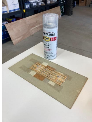
Pic 17: Coat model with clear sealant.
