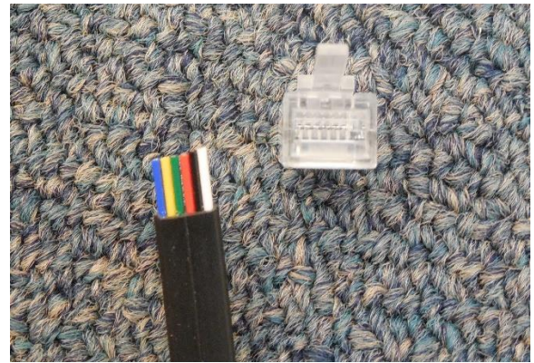
Pic 9: When assembling loconet wire runs, always keep the white wire to the right before crimping on the connector.
