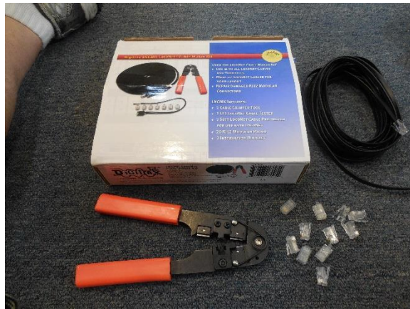
Pic 8: Digitrax Loconet set contains 50' of cable, 20 connectors, and a crimping tool.
