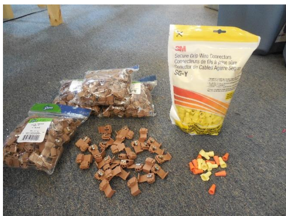
Pic 5: A variety of wire connectors are being used – easier than soldering all connections.
