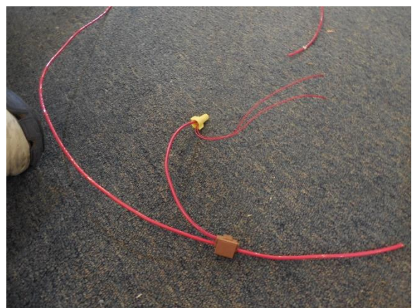
Pic 6: Feeder and drops can be pre-assembled and then connected between the bus and track.
