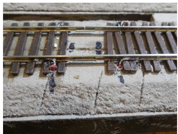
Pic 2: Feeder drops are bend to shape and soldered to every piece of track.
