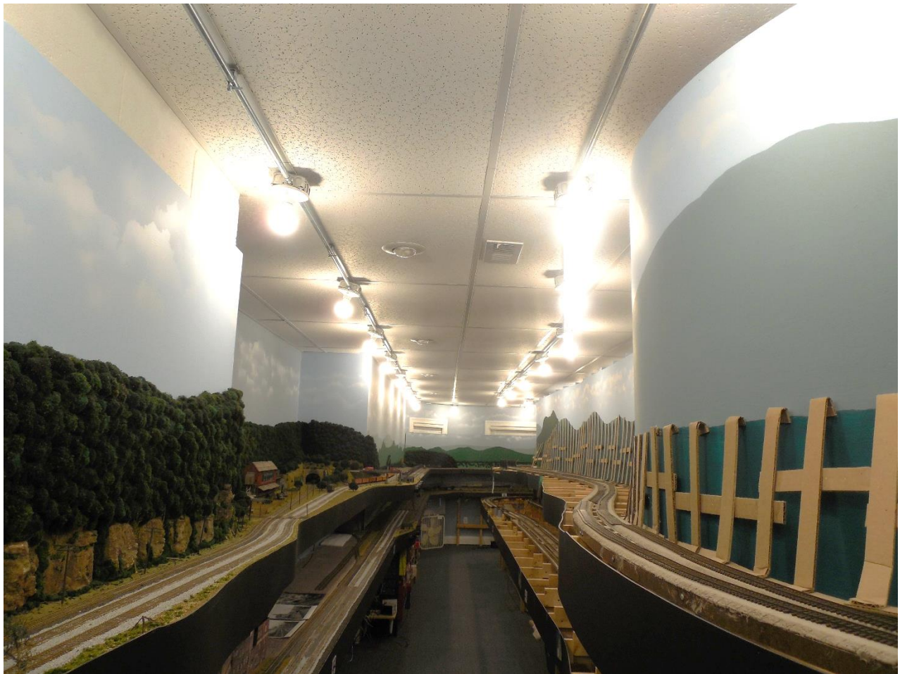
Pic 12: Lighting was changed, using LEDs instead of CFLs to avoid possible interference with Loconet signals. Next up is getting things operating.
