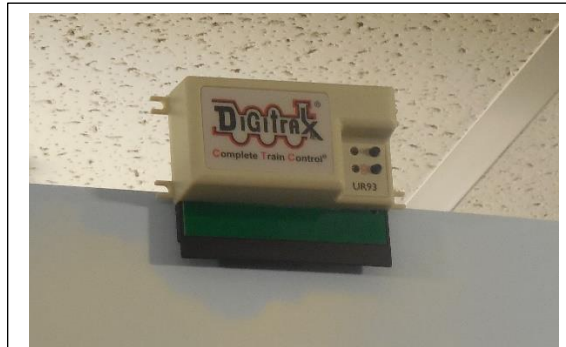
Pic 11: Digitrax UR93 for wireless communication is mounted in the center of the room at the top of the backdrop near the ceiling.
