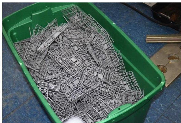
A scratchbuilder's dream. A large container catches sprues of parts as they are ejected from the high-pressure injection-molding machines.
