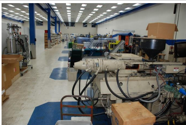
A wide range of specialized machinery is used to produce Tichy's myriad injection-molded styrene parts for kits and scratchbuilding.
