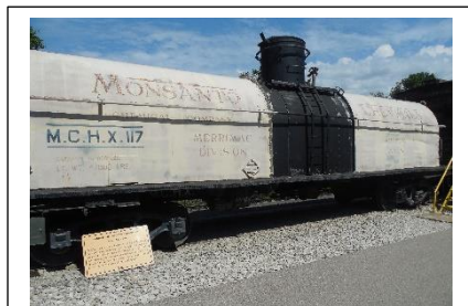
This unrestored 8,000 gallon Monsanto Chemical car dates to 1940, and has double wall construction for hauling acids.
