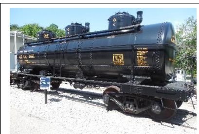
Some of the rolling stock at the museum has been beautifully restored. This three domed 6,000 gallon tank car dates to 1936.
