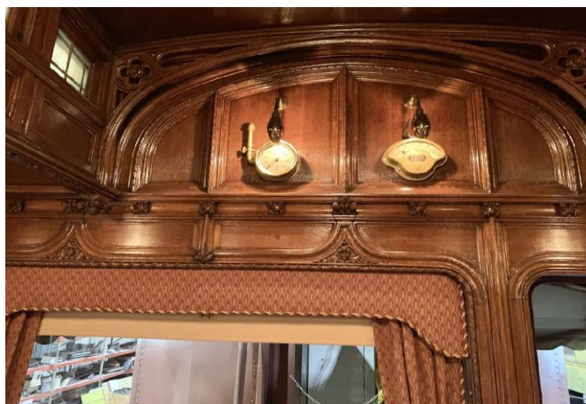
The interior of the Roamer has such beautiful gleaming finishes. Here are the train air line pressure and speedometer inside from the observation platform.
