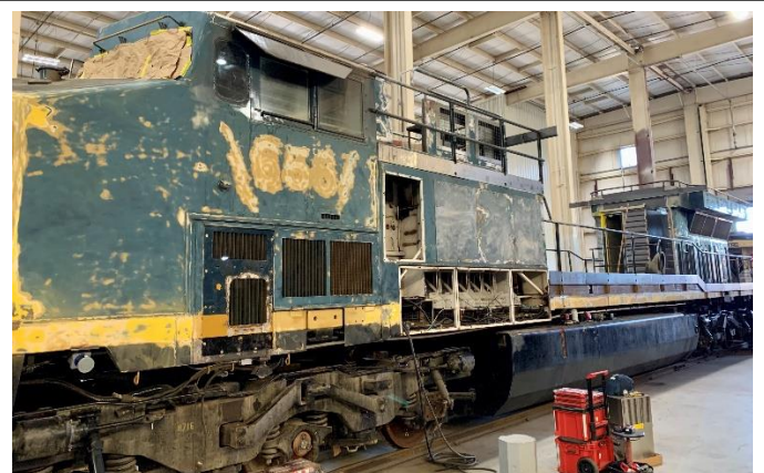
Not all effort is going into show pieces. Here a former CSX GE is undergoing an extensive rebuilding.
