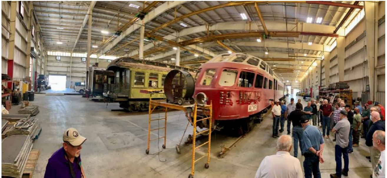
A beavertail lounge observation car from the Milwaukee Road is undergoing extensive restoration. This view is from the corner of the building. There were four parallel tracks each able to hold five cars. The shop was incredibly clean, more like a museum than a working shop.
