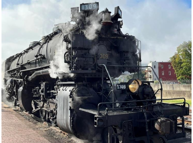
WM 1309, a compound 2-6-6-2, thus qualified to be correctly called a mallet.
