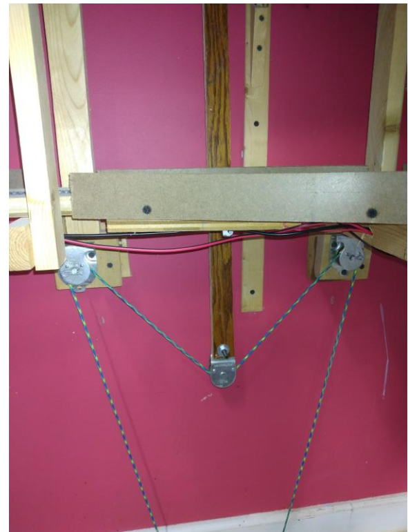
Photo 5: The actuator, center and the two pulleys mounted on each side
