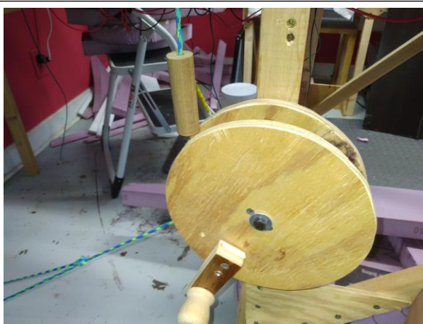
Photo 7: The Medieval reel. The rope junction with the clove hitch can be seen. This assembly was bolted to the layout leg. I turned the handle on the lathe.)
